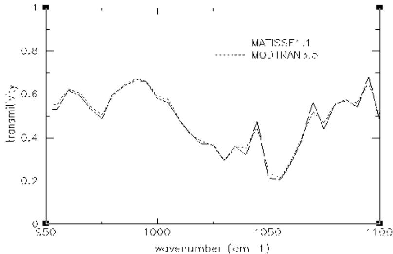
Figure 2 : MATISSE1.1 and MODTRAN3.5 total transmission comparison (molecule + aerosols)
